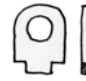
iv As for (iii), but more elongated to give a 'U' shape, with shanks of rectangular cross section
