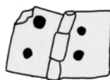
viii Square ended fixed plates, two rivets placed side by side in at least one plate
